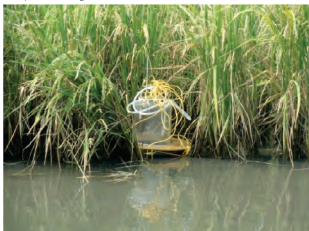
Floating chamber for the collection of GHGs in Pokkali shrimp pond
