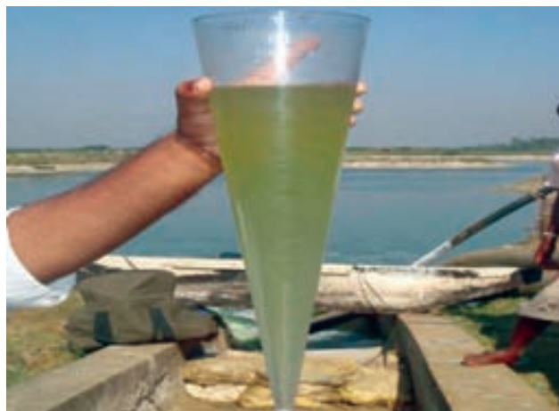
Measurement of total settleable solids at the farm site
