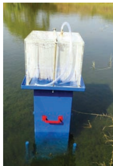
Fabricated green house gas collection sampler
