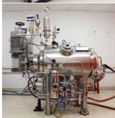
Fig. 19. Solid state fermentation of plant proteins using Aspergillus niger in pilot scale fermentor
