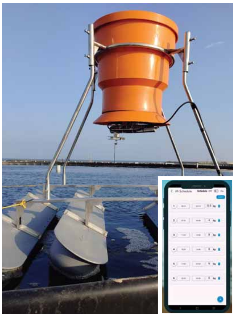
Programmed Feeding Protocols with Automated Feeders
