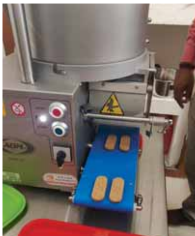
Fish patty forming machine (1000-1500 nos/hr)
